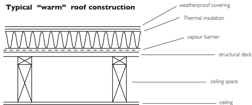
Thermal insulation material placed immediately beneath the weatherproof covering and on top of the roof deck and any vapour barrier. Deck and cavity thus maintained at warm temperatures during the winter. Condensation risk can be reduced considerably by correct selection and installation of a vapour check barrier.
