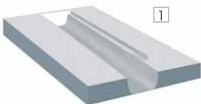
1 Adaptation of floor prior to installation
